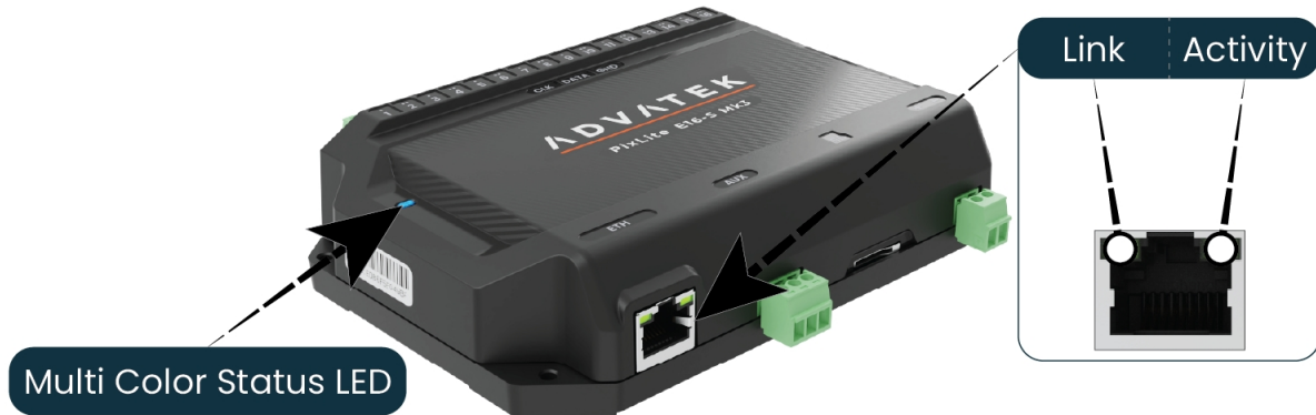
Figure 17: Location of LEDs
