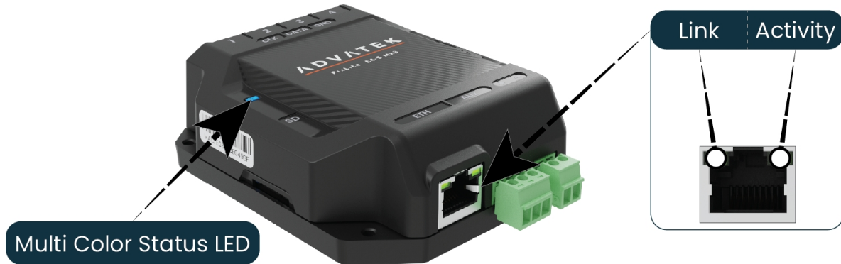
Figure 17: Location of LEDs
